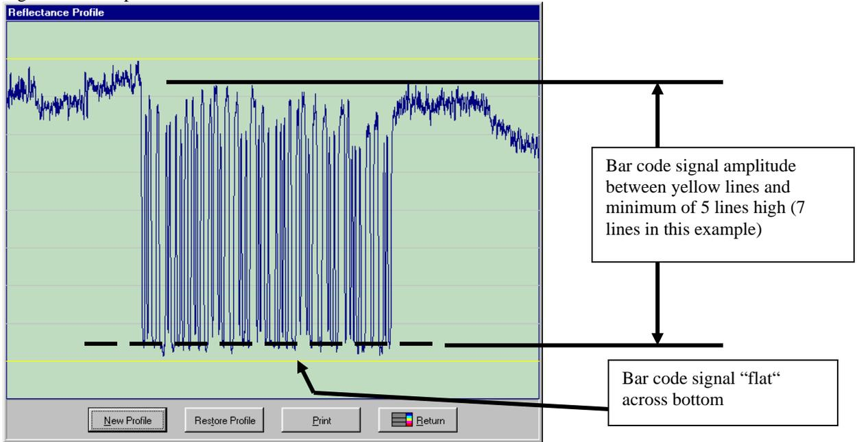
Figure 3 – Examples of Scan Profile Parameters Out of Range
