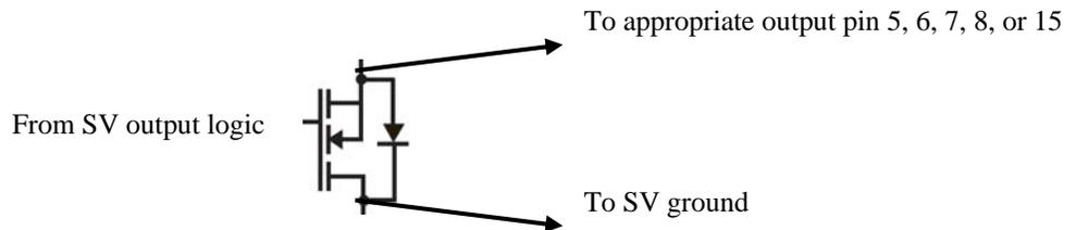
Figure C3 – Open Drain FET Output Diagram
