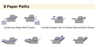
A stack of sheets with Cut Sheet Feeder and Rear Stacker(Cut Sheet Table necessary)
