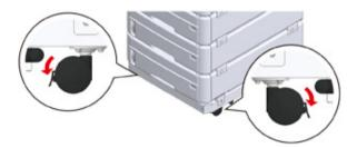
When three or more additional tray units have been attached, pull out the tipover protection tools before using the printer.
