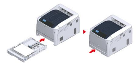
If paper that cannot be selected from the sizes on the paper size dial (the dial setting: [Other]) is loaded, set paper size to [Custom] on the operator panel and enter the width and length of paper.
