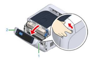
Remove the jammed paper gently in the direction of the arrow if an edge of jammed paper can be seen.
