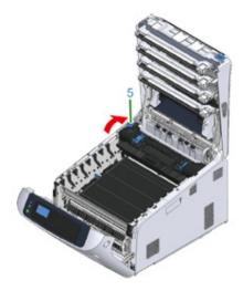
12 Return all four image drums into the machine carefully.
