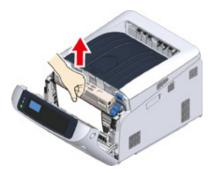
Take out the duplex unit (3) by pulling it obliquely upward while holding the center recess on the back of the machine.
