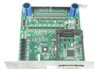
Logic Board & Power Distribution Board Assemblies
