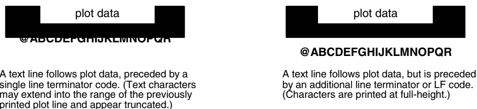
Figure 38. Truncated Character Line
