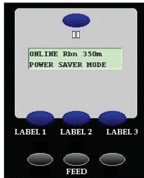
Operator Panel with GPIO Enabled
