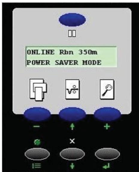
Operator Panel with GPIO Disabled
