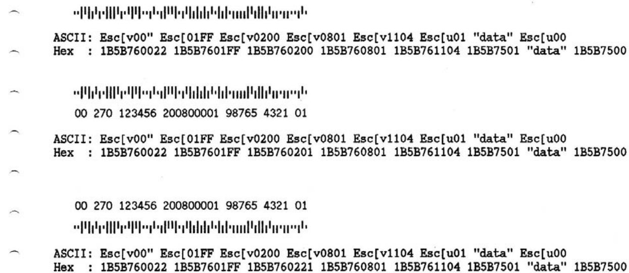
Figure 149. Intelligent Mail Bar Code in Epson/IBM Commands Example (Bar Code Mode Alt. 1)
