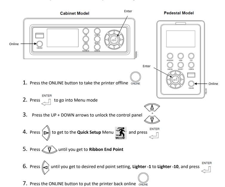
**Ribbon End Point**: This parameter adjusts the point at which the system will declare the ribbon as being expended. The life count will always be from 100% to 0%. If a lighter setting is selected the system will extend the time it takes to reach 0%. This value can be adjusted at any time, and the display will automatically adjust to show the correct % relative to the new end point.
