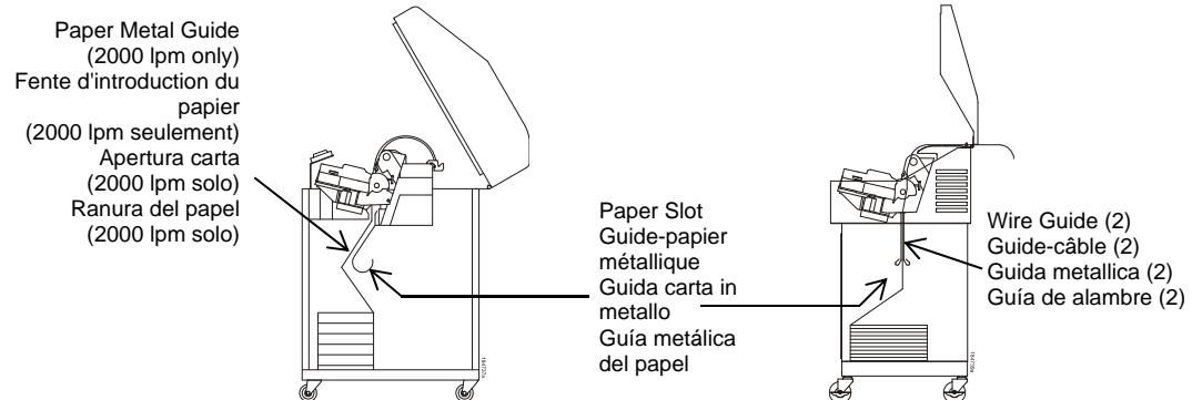
1. Align paper with label on printer floor. Feed paper up through paper slot.
