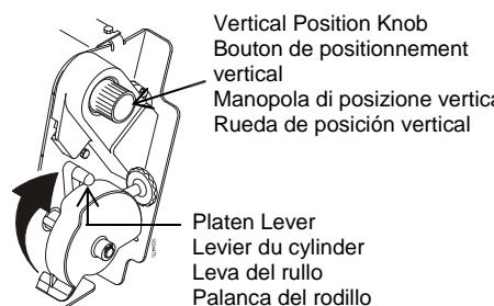
1. Ensure printer is offline. Fully raise platen lever, locate TOF indicator.
