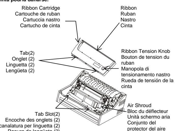
3. Hold ribbon cartridge at angle, ensuring cartridge side is lower than ribbon side. Place cartridge tabs into air shroud tab slots.
