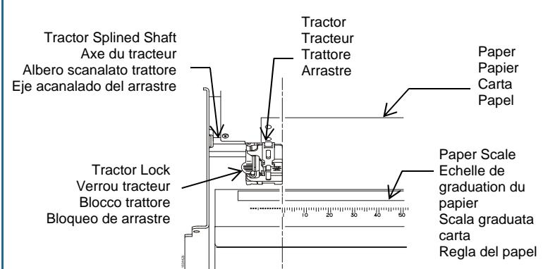
**CAUTION: Avoid platen damage by positioning left tractor to left of "1" mark on paper scale.**
