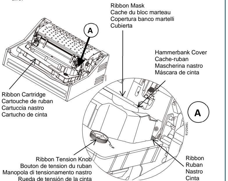
4. Rock cartridge downward, ensuring ribbon goes between hammerbank cover and ribbon mask.
