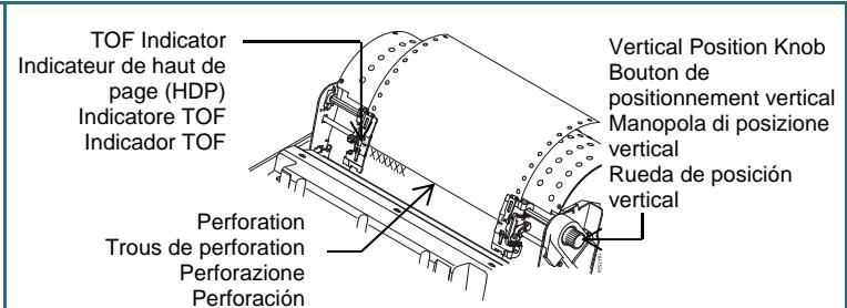
2. Turn vertical position knob to align top of first print line with TOF indicator.
